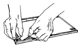
Pull firmly on tab to remove filter/light lens from range hood. Turn filter/light lens so that charcoal filter pad is facing up. Lift tabs and remove charcoal filter pad. Discard charcoal filter pad. Place edge of filter/light lens in opening so that right side is above flange and tab faces downward. Press filter/light lens into position.
